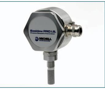
The Easidew PRO I.S. is a rugged instrinsically safe 2-wire dewpoint transmitter for trace moisture measurement in liquids and gases. It is certified for use in Class 1 Div 1 Groups A,B,C and D, EXII 1G EX ia IIC T4 and I.S. I 1 ABCD T4 (Ta = +60°C) hazardous area locations.
